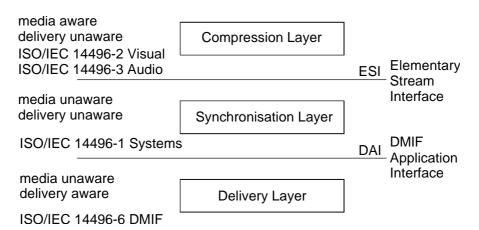
A pattern for the transport interface which enables multimedia communication over different networks and makes the application becoming independent to the delivery architecture was defined. The next figure shows the architecture of an MPEG-4 communications solution for different network structures.
